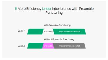
Preamble puncturing identifies and excludes interference-affected subcarriers, reducing spectral waste and boosting efficiency in challenging wireless conditions.
