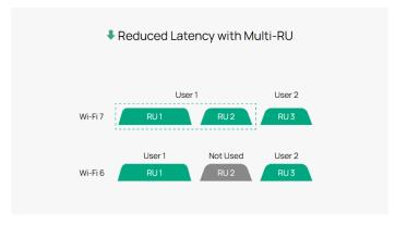
Wi-Fi 6 restricts each user to a single resource unit (RU), limiting spectrum flexibility. Wi-Fi 7 overcomes this limitation by allowing multiple RUs to be allocated to a single user and enabling RU aggregation, improving data throughput and spectral efficiency.
