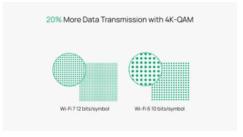
$4096\text{-}QAM\ enables\ each\ symbol\ to\ carry\ 12\ bits\ instead\ of\ 10,\ increasing\ theoretical\ transmission\ rates$  by 20% compared to Wi-Fi 6's 1024-QAM. This higher transmission rate boosts\ data\ throughput, delivering\ enhanced\ speeds\ and\ improved\ network\ reliability.
