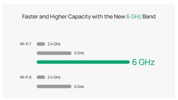
The new 6 GHz band offers a larger spectrum and cleaner channels compared to traditional bands, delivering higher capacity, faster connectivity, and less interference.
